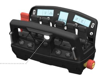
The centre display is the system's information centre. It shows information that is not directly related to the crane's operation.
