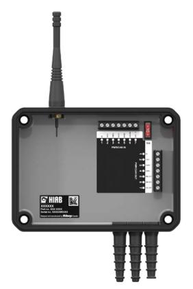
For safety reasons, it is extremely important that data is not corrupted, therefor the decoder has dual micro-processors which monitor each other to ensure accuracy in the translation. The controller and the decoder must be "paired" with each other to establish a connection. A unique code is loaded and stored in each unit. The pairing procedure is described elsewhere in this documentation.
