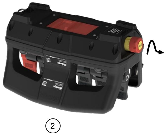
Connection time for a cold-start can be up to 5 seconds. A cold-start occurs when the hand controller or decoder on the crane have been off for the last 10 minutes. When restarting within 10 minutes of turning off the hand controller, the radio link is still established and the hand controller is ready for use immediately.
